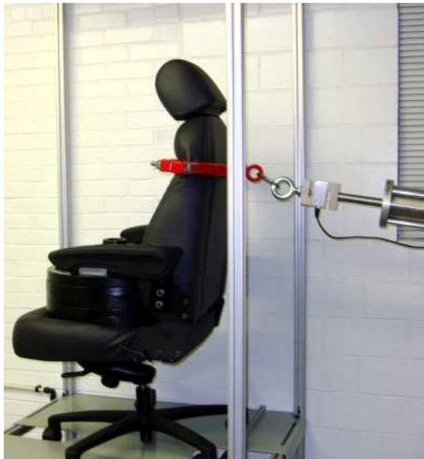
PICTURE 5: TILT MECHANISM TEST - CYCLIC
