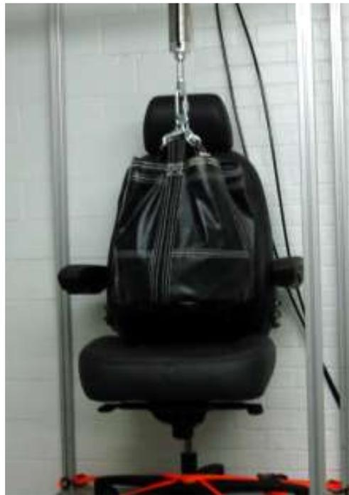
PICTURE 6: SEAT DURABILITY IMPACT TEST - CYCLIC
