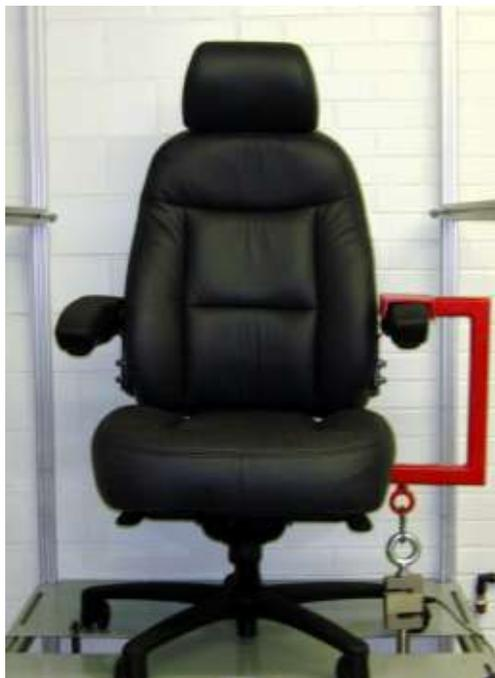
PICTURE 10: ARM STRENGTH TEST - VERTICAL - STATIC
