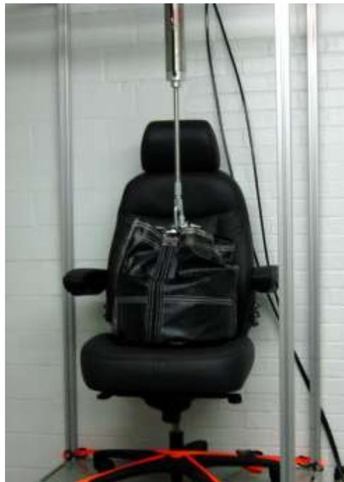
PICTURE 3: DROP TEST PROCEDURE
