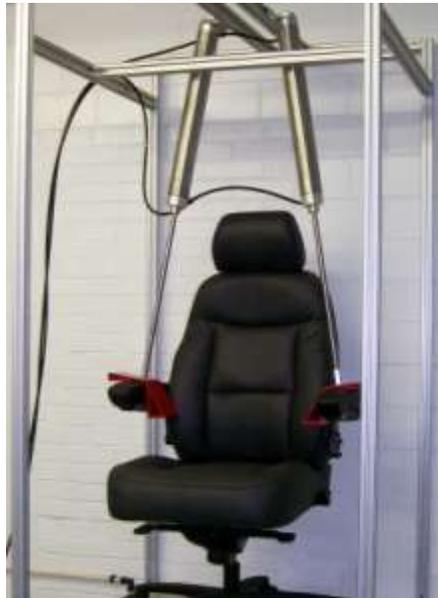
PICTURE 14: ARM DURABILITY TEST - CYCLIC
