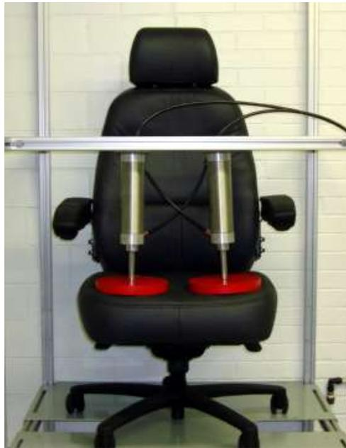
PICTURE 7: SEAT DURABILITY LOAD EASE TEST - CYCLIC
