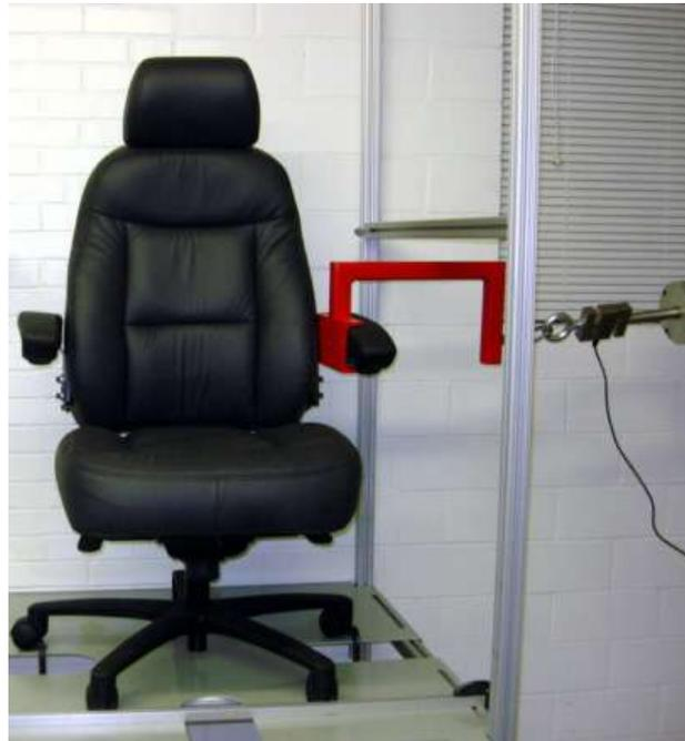
PICTURE 11: ARM STRENGTH TEST - HORIZONTAL - STATIC
