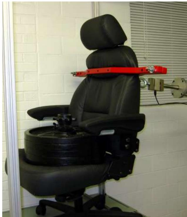
PICTURE 12: BACKREST DURABILITY TEST - CYCLIC - TYPE 1
