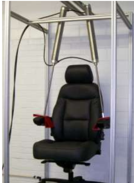
PICTURE 14: ARM DURABILITY TEST - CYCLIC
