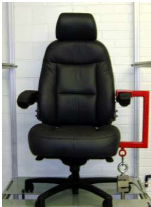
PICTURE 10: ARM STRENGTH TEST - VERTICAL - STATIC
