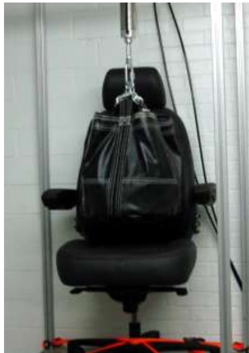
PICTURE 6: SEAT DURABILITY IMPACT TEST - CYCLIC
