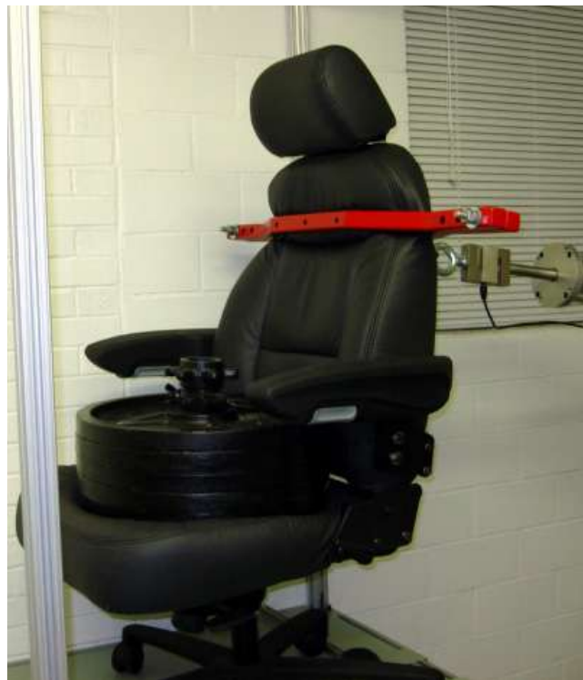
PICTURE 12: BACKREST DURABILITY TEST - CYCLIC - TYPE 1
