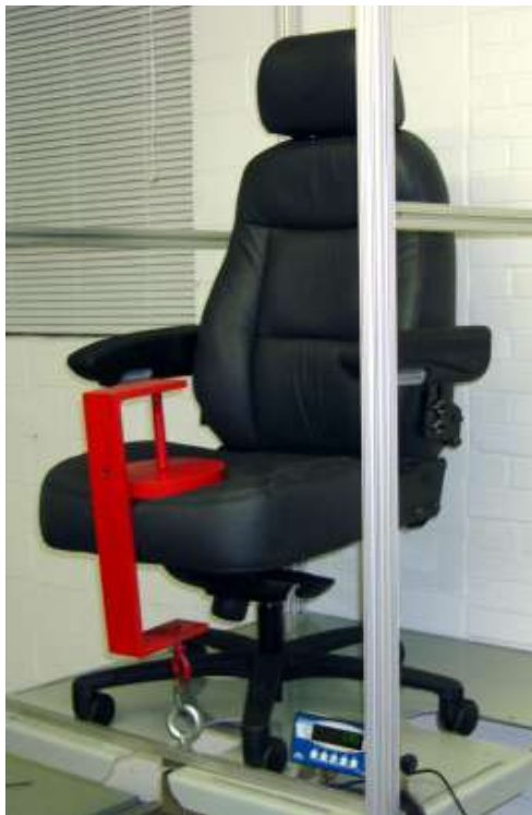
PICTURE 8: FRONT STABILITY TEST
