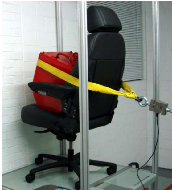
PICTURE 9: REAR STABILITY TEST
