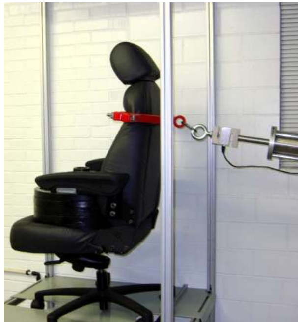
PICTURE 5: TILT MECHANISM TEST - CYCLIC
