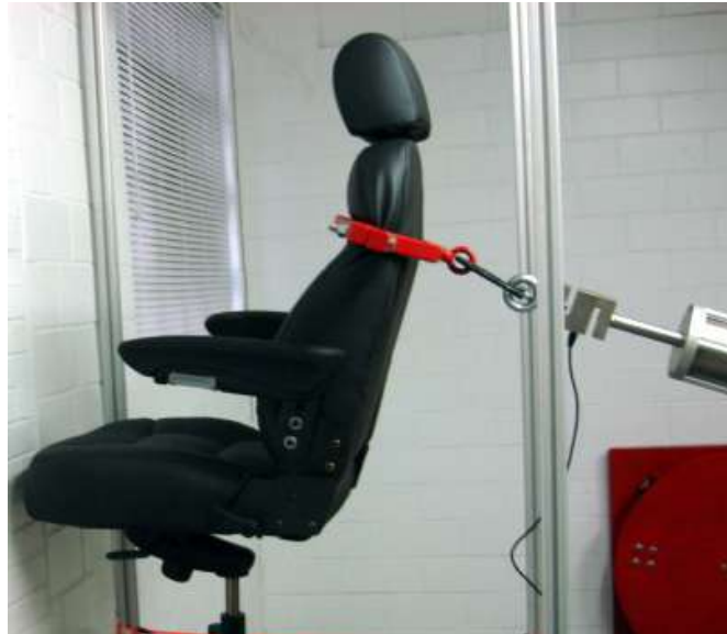
Picture 1: Back Strength Test Procedure
