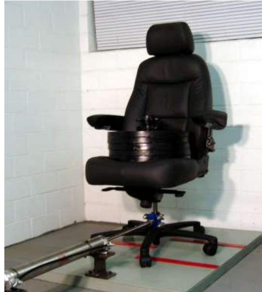
FIGURE 13: CASTER / CHAIR BASE DURABILITY TEST - CYCLIC
