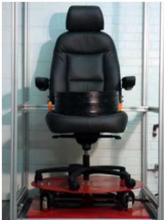
PICTURE 4: SWIVEL TEST - CYCLIC
