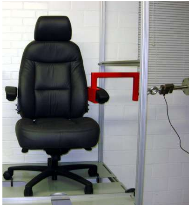
PICTURE 11: ARM STRENGTH TEST - HORIZONTAL - STATIC
