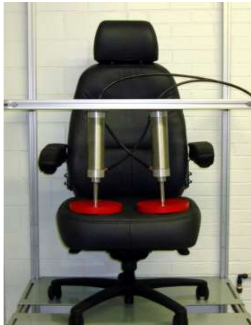
PICTURE 7: SEAT DURABILITY LOAD EASE TEST - CYCLIC
